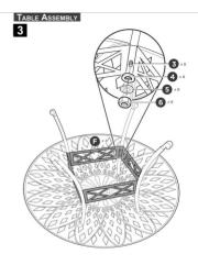
Attach four part F supports to the table legs with eight part 3 fastener, eight part 4 washers, eight part 5 spring washers, and eight part 6 nuts.
