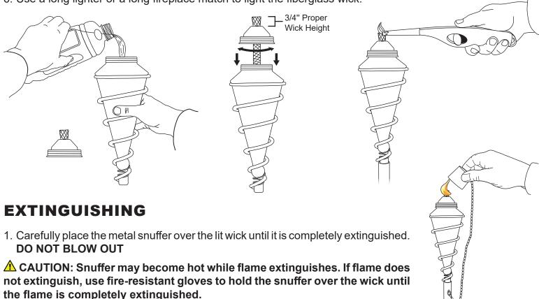
**IMPORTANT:** When the torch is not in use, leave the snuffer on the torch to prevent water contamination. If the fuel becomes contaminated with water, the wick and fuel must be replaced. Torch fuel must be properly disposed of in accordance with local laws and regulations.
