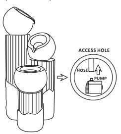
**2.** Extend the pump and LED light cables through the access hole in the back of the fountain, cables are ready for connection to the solar panel.
