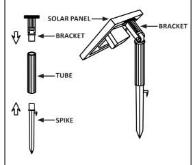
**5.** Insert the spike into the ground. Position the solar panel to face south (in the northern hemisphere) to make the most of daylight hours. It is important to angle the solar panel towards the sun when the sun is at its highest point. Ensure trees, shrubs, or buildings do not shade the solar panel.
