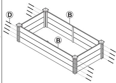
Align Side Panels (B) between the corner posts of the assembled components.
