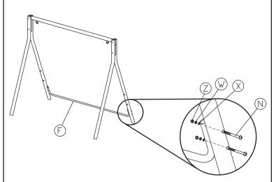
Connect Back Support (F) to Back Legs (B) using Bolts (N) and M6 hardware (X+W+Z).
