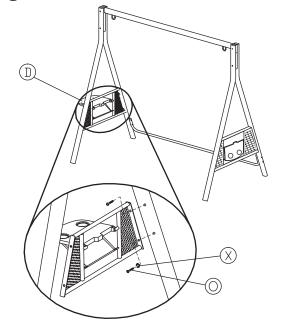
· Fasten Side Table Panels (D) to the front and back legs using Bolts (O) and M6 Washers (X).
