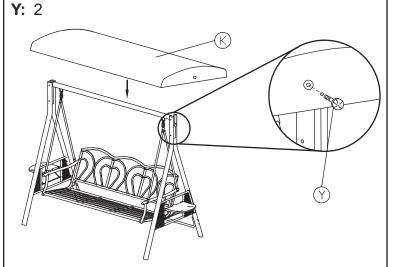
Open Canopy (L) and align the holes of the canopy frame with the swing frame. Secure the canopy to the frame using Threaded Knobs (Y).
