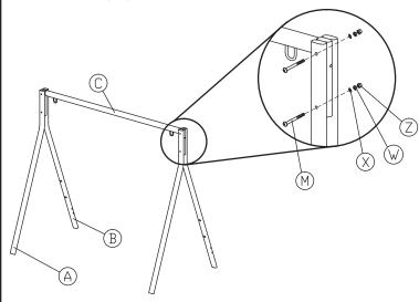
Attach Front Leg (A) and Back Leg (B) to Top Bar (C) using Bolts (M) and M8 hardware (X+W+Z).
