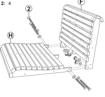
Do not fully tighten hardware until Step 6 is complete.
