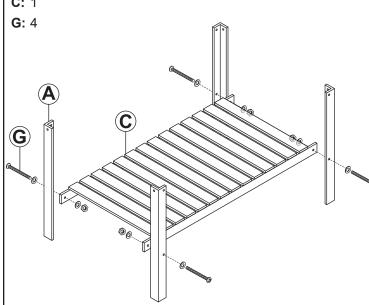
Attach 4x Leg (A) to Shelf (C) by hand-tightening 4x M6x40mm Bolt Set (G), as shown.
