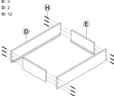
Ensuring the lipped edges on the bottom, align Side Panel (D) with End Panel (E) and firmly secure using 3x Screw (H). Repeat until planter box frame is assembled.
