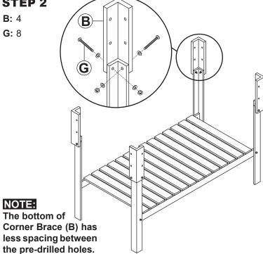
Align the bottom hole of Corner Brace (B) with the outside of Leg (A). Secure by hand-tigtening 2x Bolt Set (G). Repeat to connect remaining corner braces. Do not over-tighten hardware.
