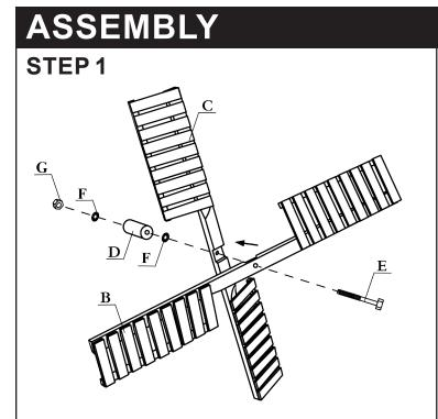
Place Front Blade (B) onto Back Blade (C) as shown. Slide Bolt (E) through the blades, Washer (F), Shaft (D), Washer (F), and Nut (G). Hand-tighten the bolt. **Do not over-tighten the hardware.**
