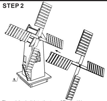
Thread the bolt into the top of Tower (A).
