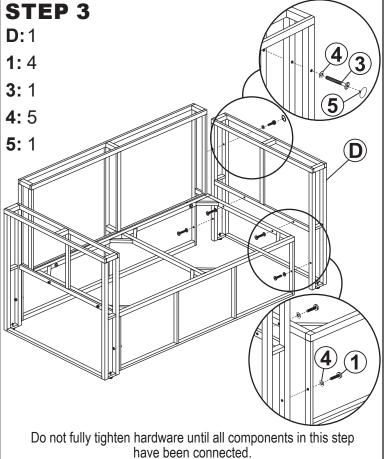
Do not fully tighten hardware until after Step 3 is complete.
