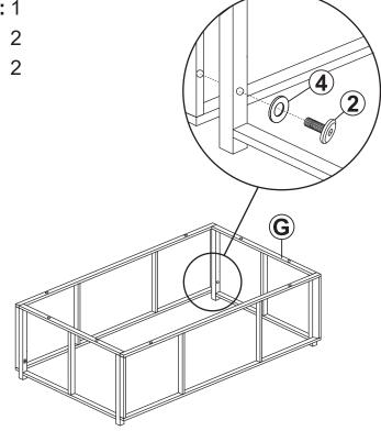
Do not fully tighten hardware until after Step 11 is complete.
