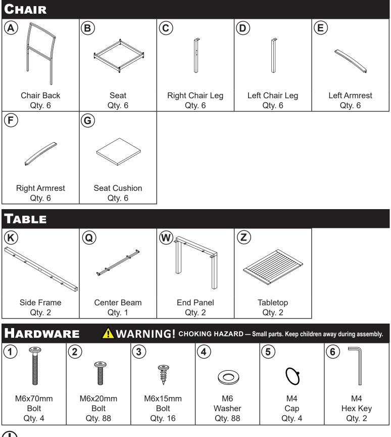
**HELPFUL HINT:** Do not tighten hardware until all components have been loosely assembled. If the hardware is tightened too soon, mounting holes may not align, and parts may not easily fit together.
